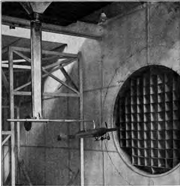
Fig. 36. Method of Testing Models of the Eiffel Aerodynamometric Laboratory
